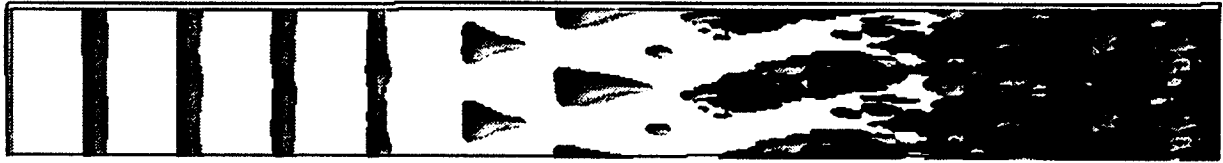
Figure 15 Same as Figure 12, without the iso- |\omega_{x_1}| surface, replaced by isosurface \nu_t = 0.33\mu_\infty/\rho_\infty given by the FSF 3 model, (dark gray)
